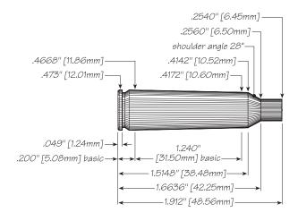
Max. Case Length:1.912"Cart. Case:Federal®Trim-to Length:1.902"Primer:Federal 210Max Cart. OAL:2.350"Test Firearm:Universal ReceiverRCBS® Shell Holder:#3Barrel Length:24"
